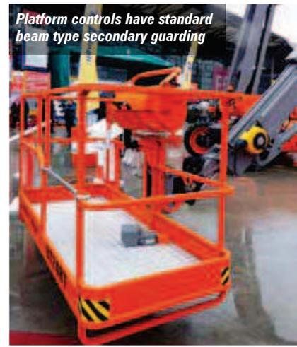
*Platform controls have standard beam type secondary guarding*
