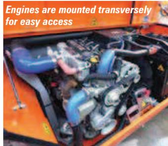
Engines are mounted transversely for easy access
