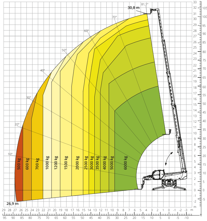
Load chart with FULLY EXTENDED STABILISERS (360°) ATT-03-004
