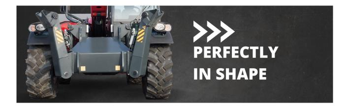
Both models are equipped with a +/- 8° levelling system on tyres that allows the operator to adjust the machine's inclination and to have the full load chart in all operations, even on irregular terrain that would normally compromise lifting performance.
