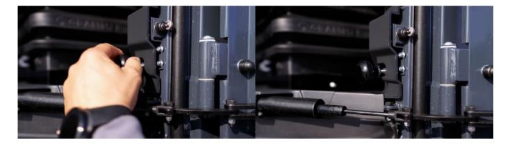
Magni's patented "**easy access**" system automatically stops the turret rotation when approaching the access ladder, simply by pressing a green button on the left joystick.
