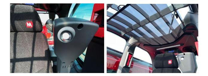
Airflow inside the cab has been improved with a new design in the lower part of the windscreen to optimise defrosting in cold weather.
