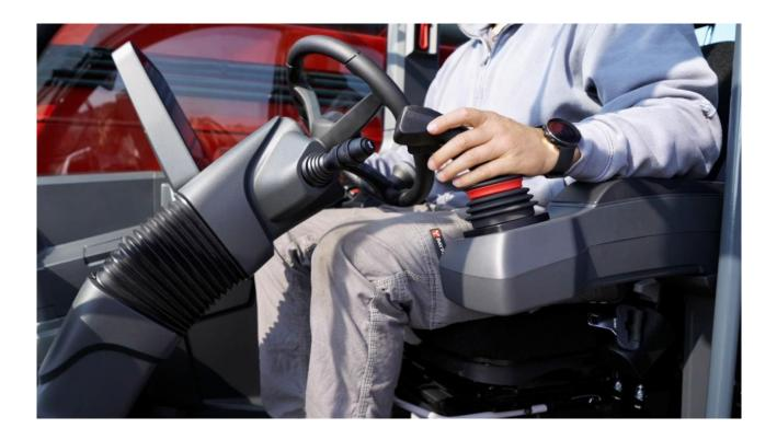
In the new cab, the two **armrests** on the seat (which can also be adjusted independently) can now be raised to create a practical storage compartment under the right armrest. In the upper part of the cab, two technical compartments have been fitted to house most of the electrical control units, fuses and diagnostic sockets to facilitate routine and extraordinary maintenance.
