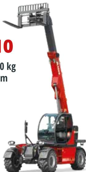
Deutz 100 kW (136 CV) a 2200 rpm
