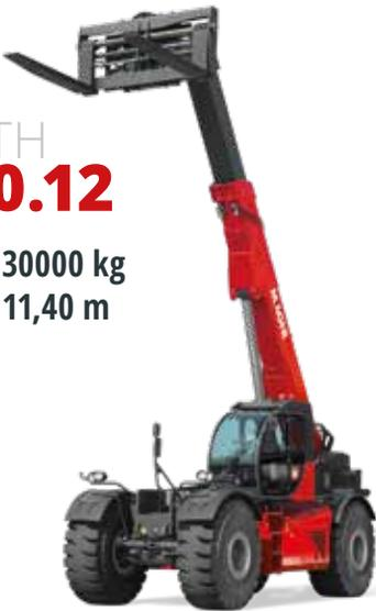
Volvo 235 kW (320 CV) a 2200 rpm
