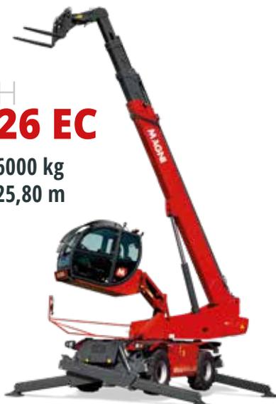
Deutz 100 kW (136 CV) a 2200 rpm
